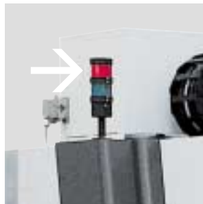
Optical operating indicator Light column that optically indicates the operating status of the machine.
