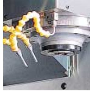
Minimal lubrication A minimal lubrication system with two nozzles that specifically applies a microfilm of lubricant, which covers the cutting edge of the tool with high flow speed.
