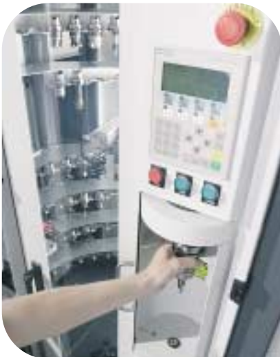
Circularly arranged magazine with a handling system for 75, 120, 170 or 220 tools.
