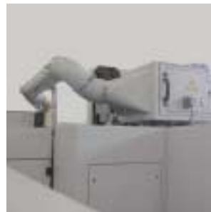
Mist exhauster A compact, electrostatic aircleaner with multiple levels of filtration that is specially adapted to the filtration of oil and emulsion mist.
